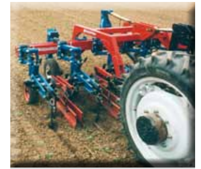
6-row sugarbeet hoe use in small sugarbeet plants with protection plates
