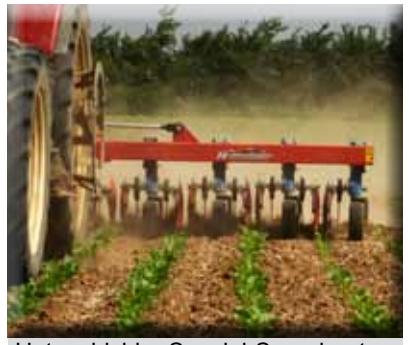
Hatzenbichler Special-Sugarbeet hoe, 12-row with planting protection discs
