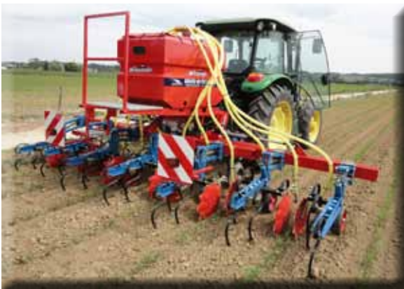
6-row rear-mounted with mounted pneumatic fertilizer spreader in working position and crop protection discs. Fertilizer box with 1000 kg Capacity.
